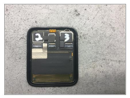
Yup, that's our Series 2 Display with the NFC module from the broken S3 Display attached. Alignment here is fairly important so don't just slap it on all willy-nilly.
