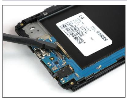
Disconnect the display flex cable with the flat end of a spudger.
