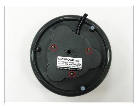
screw down three screws off in the middle.
