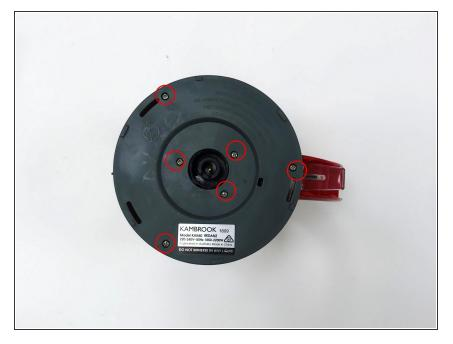
• Turn the device upside down and screw down the screws.
