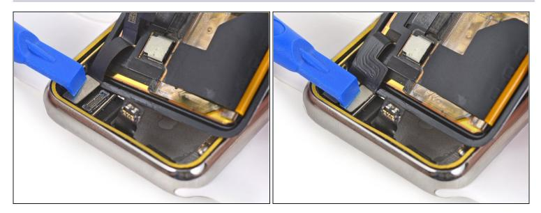
• Use a plastic opening tool to reconnect the display data and digitizer cable connectors.
