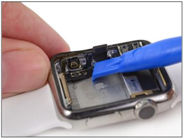
• Use a plastic opening tool to flip the Force Touch sensor cable connector straight down, disconnecting it.
