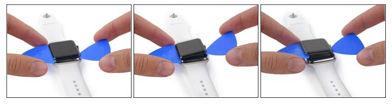
There are two cables connecting the screen to the inside of the watch, near the top left corner. Be careful when prying or you may damage these cables.
