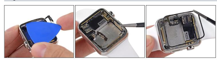
• Use a plastic opening pick and <u>tweezers</u> to remove the Force Touch sensor from the case.
