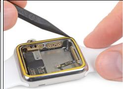
• Gently but firmly press the Force Touch sensor into place all around the perimeter of the watch case.
