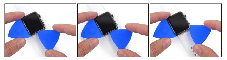
• While holding the first pick in place, use a second to check that all of the adhesive is separated around the entire perimeter of the screen.
