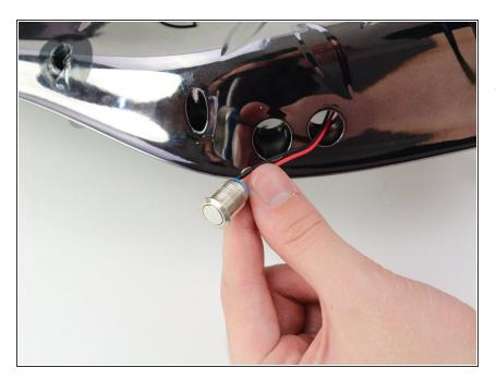
Feed the wire and connector through the removed nut and pull the power button out through the hole in the outer casing.
