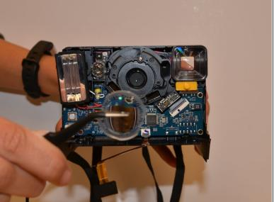
Remove the clear plastic lens with tweezers.
