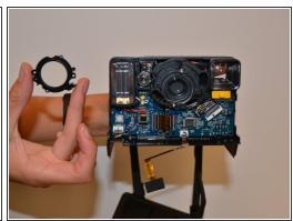
Remove the two Phillips #0 3mm screws on the black ring holding the lens in place and remove the ring.
