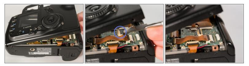
Mhen lifting the panel, make sure not to lift it too high, since you'll run the risk of tearing the cable, or damaging the connector on the board.
