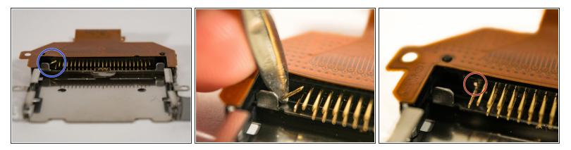
• This is one of several issues with this CF connector. This pin is severely bent.
