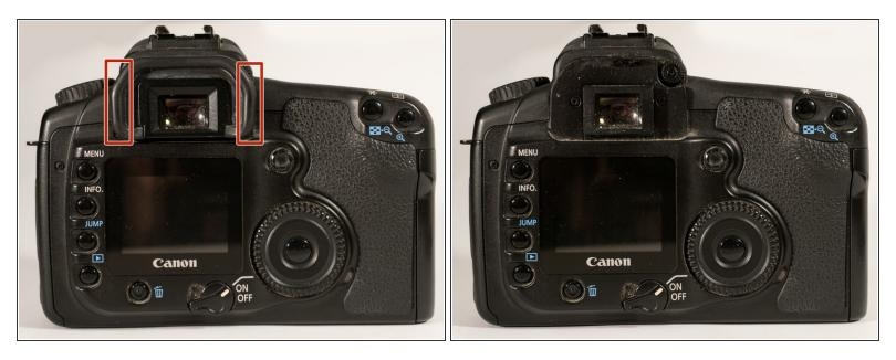
Pull up on both sides of the the eyepiece cap. It should come off with little pressure.
