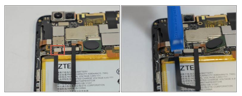
• Using a plastic opening tool, separate the fingerprint ribbon connector from the motherboard.
