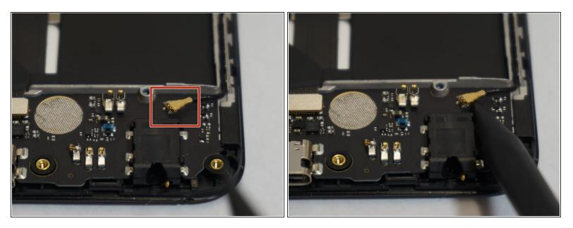
• Use a spudger to pry up the the antenna connector on the top right of the charging port card.
