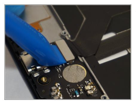
Use a plastic opening tool to pry up and remove the primary connector for the card, located on the top left of the card.
