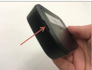
Hold the device with your non-dominant hand, looking at the back of the device, taking note of the small notch along the edge.
