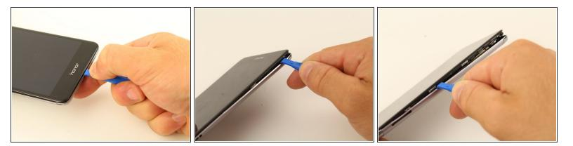
• Slide the opening tool or spudger along the bottom of the phone and around the edge.
