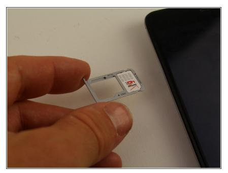
• Remove the SIM card from the compartment using two fingers.
