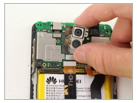
• Gently remove the camera assembly using a spudger or two fingers.
