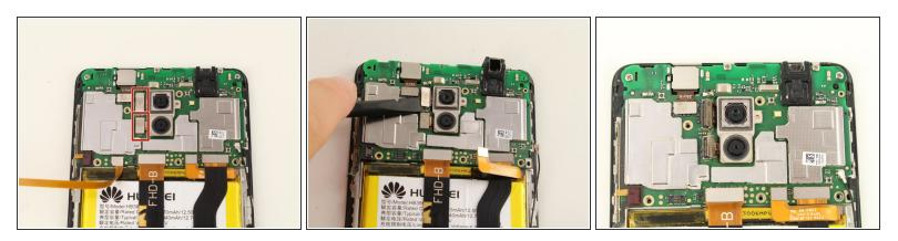
• Pry the two connectors off by wedging a spudger, or your finger, underneath the connector.
