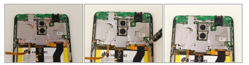
• Remove the five 4mm Phillips #00 screws using a screwdriver.
