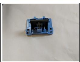
Now with both screws out, remove the paper feeding housing from the printer.
