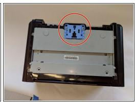
Flip printer on its back to expose the paper feeder housing.
