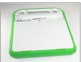
Lift the middle of the battery to remove it.
