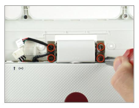
Using the Phillips screwdriver, unscrew the 4 size M3 x .5 x 5mm screws holding the metal to the rest of the laptop.
