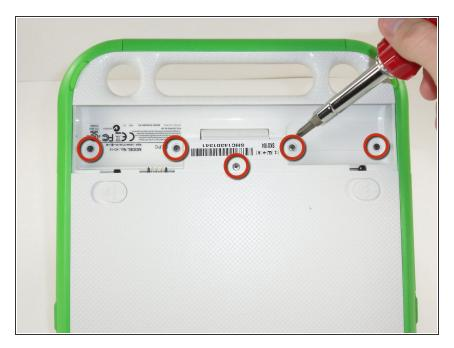
Using the Phillips screwdriver, unscrew the 5 size M2 x .4 x 4mm screws underneath the battery.
