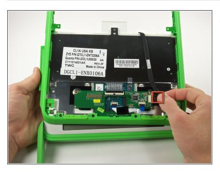
Slide the black cable (the one that holds the two halves together) out of its connector.
