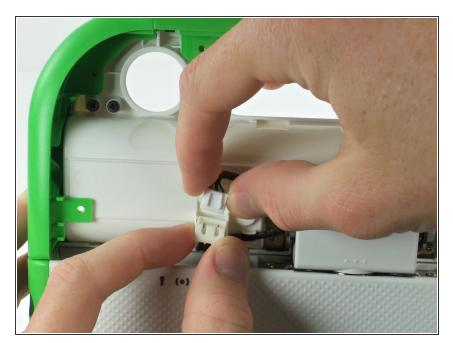
Unplug the white connector with black cables on each end on the left of the hinge.
