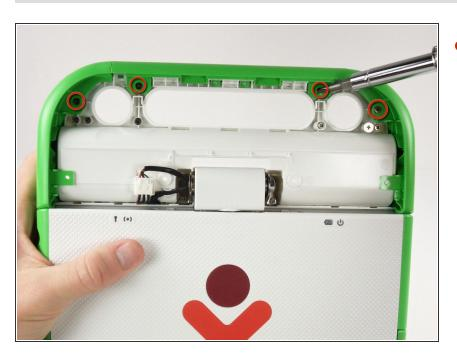
Unscrew the 4 size M2 x .4 x 4mm screws that are connected to the green plastic.
