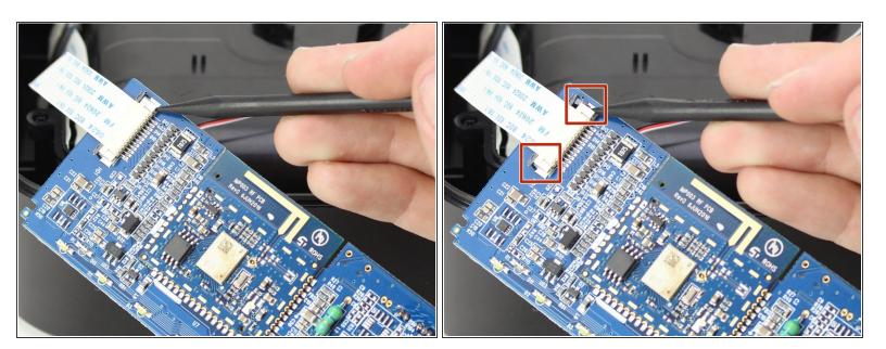
Push both small gray pieces next to the ribbon connector towards the ribbon to put them in the "open" position using the nylon spudger.
