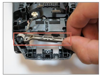
Remove the front vision piece by pulling the piece up and away from the drone body.
