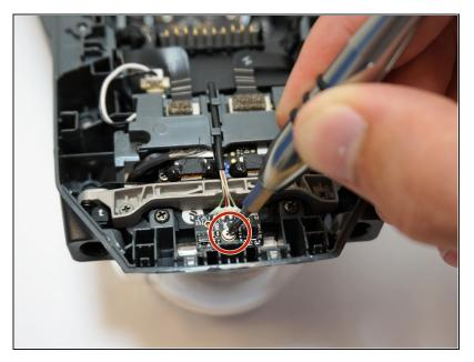
Remove the one 5mm JIS #0 screw from the small micro controller board at the front of the DJI Mavic Pro by turning counterclockwise.
