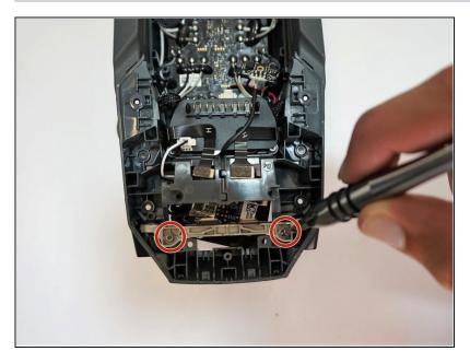
Remove the two 6mm JIS #0 screws by turning counterclockwise.
