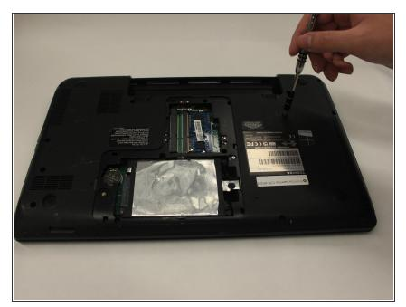
Using the PH1 screwdriver, remove the remaining screws from the back casing of the laptop.
