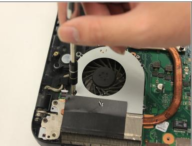
Remove the 2 screws holding the fan in place.
