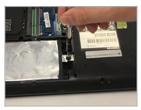
Remove the screw next to the hard drive using the PH1 screwdriver.
