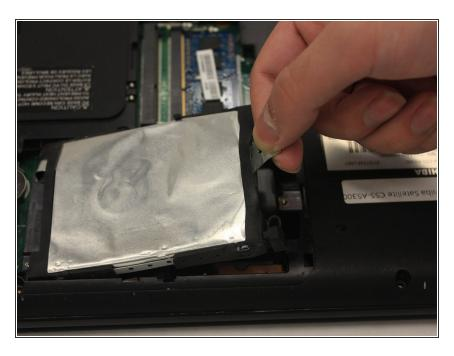
Pull the silver tab connected to the hard drive up to take it out.
