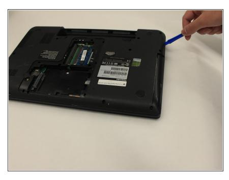
Use a nylon spudger or plastic opening tool to carefully wedge the casing apart and remove the back plate of the laptop.
