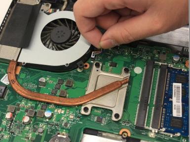
• Detach the multi-colored wire connecting the fan to the motherboard and pull the fan out.
