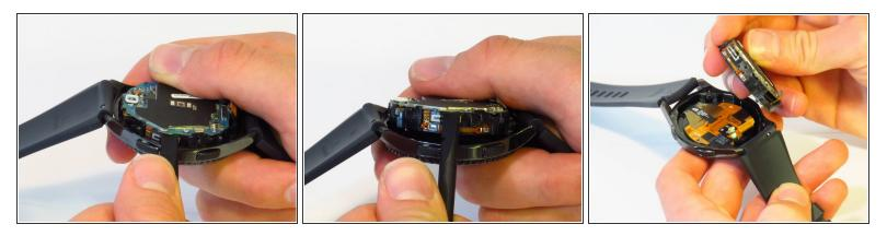
• Separate the motherboard and front screen assembly using a spudger.
