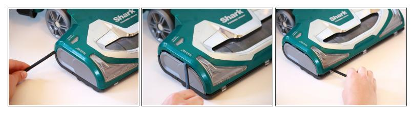
Flip the vacuum into the upright position, and use a spudger to open the front assembly cover by prying the seam where the colored front assembly and the grey side covers meet.
