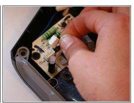
Pinch the tabs on the circuit board clasp for the LED headlight inwards, and pull the clasp up and away to detach the headlight.
