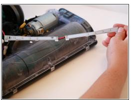
Pull the LED headlight strand up and away from where it is attached to the bottom front of the vacuum.
