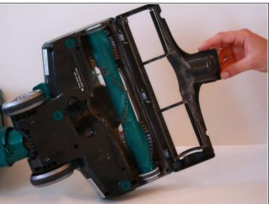
Squeeze the sides of the roller brush cover release clasp, and swing the cover open.
