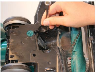
Using a T20 screwdriver, remove three 13.4 mm screws from where the roller brush cover attaches to the bottom of the vacuum.
