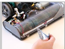
• Use a spudger to remove the headlight covers by prying the seams where the headlight covers meet the bottom front of the vacuum.
