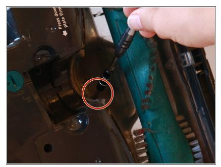
Using a PH0 screwdriver bit, remove the single 13.4 mm screw in between the roller brush and where the release clasp was attached.
