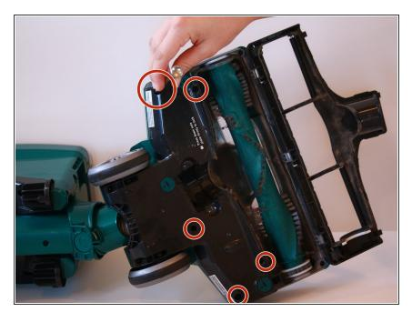
Using a T20 screwdriver remove five 15.9 mm screws on the outside of the cover.
