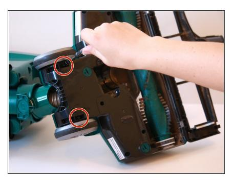
Using a T20 screwdriver, remove two 13.4 mm screws from under the wheels.
