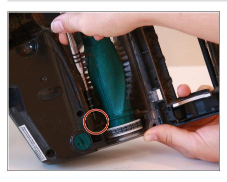
Using a T20 screwdriver, remove the single 13.4 mm screw from behind the belted end of the roller brush.
