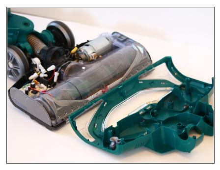
Separate the front assembly cover from the vacuum.
