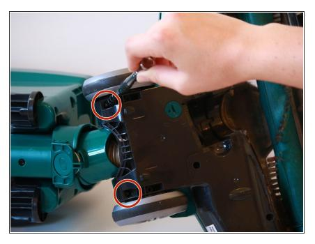
Using a T20 screwdriver, remove two 15.9 mm screws behind the vacuum wheels.
