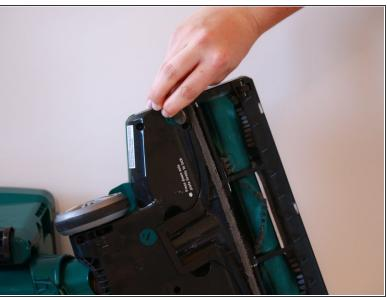
• Flip the vacuum on its underside, and use a coin to rotate the cam-screws on the bottom panel so that their grooves are parallel with the front of the vacuum.
