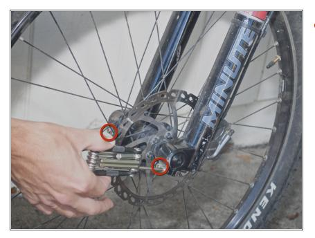
Using the 4mm Allen wrench, partially unscrew the 4 (22mm) hex screws on the front of the axle casing to allow the axle to slide freely.
