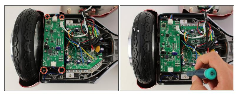
• Remove the four 11mm Phillips #1 screws that hold the cover on.
