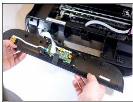
Slide the front panel to the right, then lift the front panel upwards.
