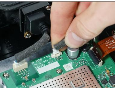
Unplug the optical audio port from the main circuit board by pinching the white clip and pulling upward.
