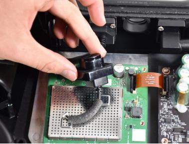
Remove the Optical Audio Port from the housing by pinching the sides and pulling outward.
