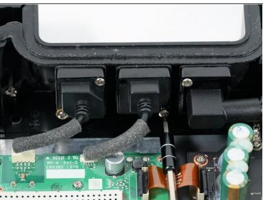
Remove the two 18mm <u>T-10</u> screws holding the Ethernet Port in place by turning them counterclockwise.
