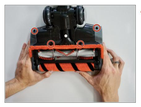
Remove the four 15 mm T10 screws on the underside of the vacuum.
