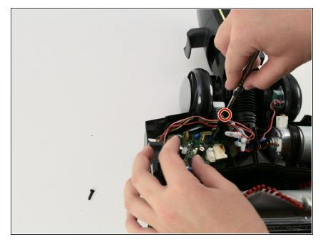
Remove one 15mm T10 screw from the inside left of the base of the vacuum to access the motherboard.
