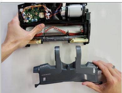
Using the plastic spudger, pry the back seam of the top component to pop it off the vacuum.
