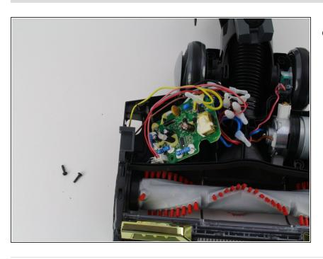
Desolder the motherboard wires using wire cutters.
