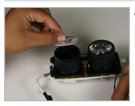
Holding the lens around the outside, gently lift it out of its housing.
