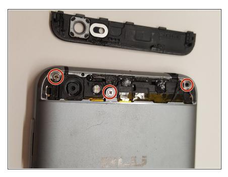
Using a Phillips #000 screwdriver, remove the 3mm screws. Be sure to do this for the top and bottom of the phone.
