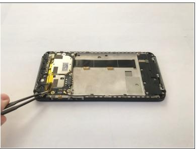
Remove the yellow plastic tape using a pair of tweezers.
