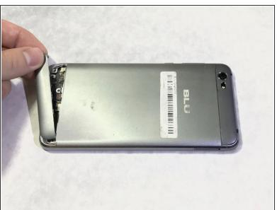
Remove the two plastic plates with a plastic opening tool.
