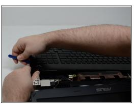
Pry around the keyboard on the top topside as shown to remove it from shell.
