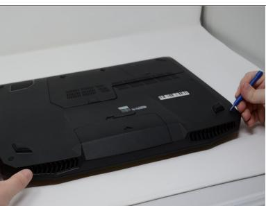
Using a plastic opening tool, remove the two rubber tabs circled in red.
