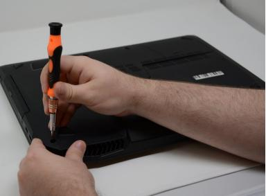
Remove both of the 8mm Phillips #2 screws from these slots where the rubber caps were removed.
