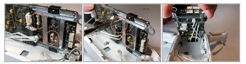
• Lift up or tilt entire frame and mother board and unplug all the wires.
