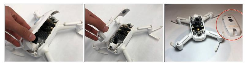
• Grip the cover that covers the rest of the wires, and give it a slight pull to remove it.
