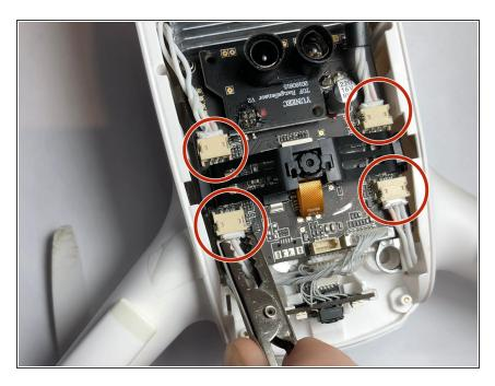
Unplug the four cables that are connected on the top face of the frame.
