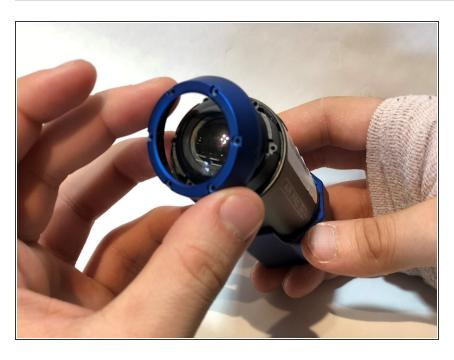
Lift the lens cover bezel off of the camera body.
