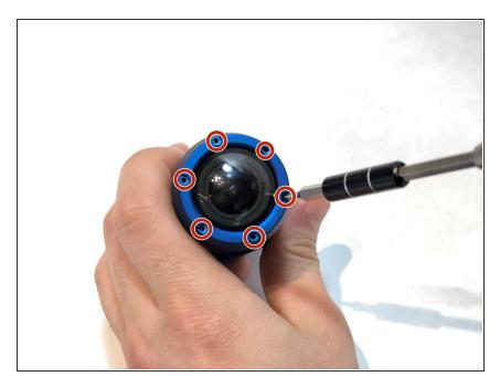
Remove the 6 screws that secure the lens cover bezel with a #00 Phillips screwdriver.
