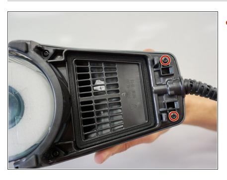
Remove the two 15 mm screws by twisting counterclockwise with the T10 Torx screwdriver.
