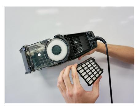
Remove the post-motor filter.
