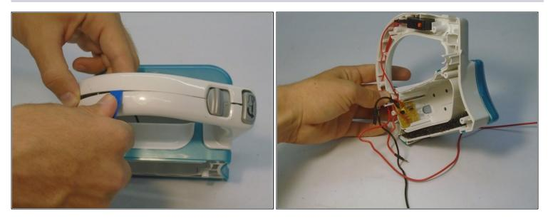
• Use a plastic opening tool to separate the two pieces of plastic.
