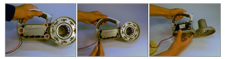
• Remove the three screws highlighted with red circles.
