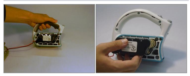
• Remove the battery by pulling it out of the slot it sits in.
