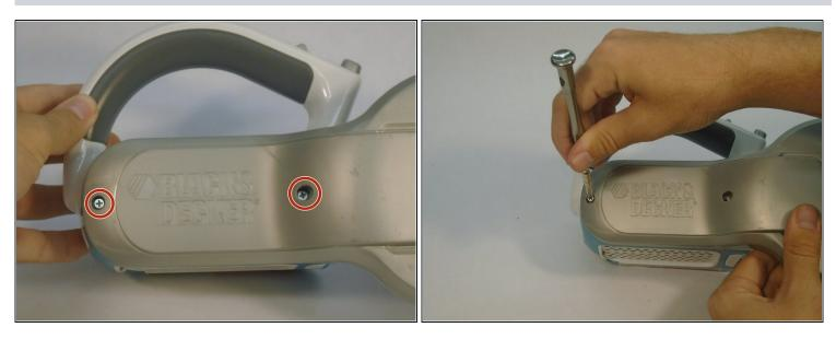
• Flip the hand vac over and remove two screws.
