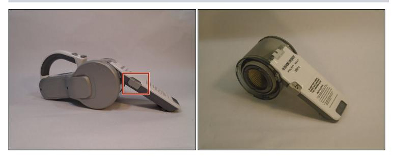
To take off the nozzle, filter, and catch bowl first start off by pushing in the button identified with a red square and twist that part of the device toward the handle portion of the vacuum and it should click and pop off the chassis.
