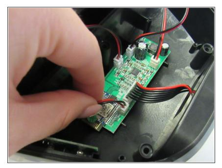
Detach the wiring piece, located in the upper right corner of the motherboard.
