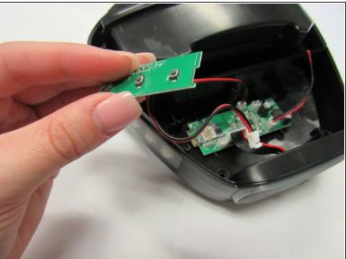
• Remove the daughterboard piece from its designated slot, located to the right of the motherboard.
