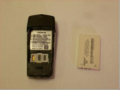
Use a screwdriver or spudger to lift the battery out of the casing.
