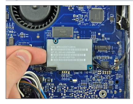
• Use your finger to lift the AirPort/Bluetooth board from its left edge, disconnecting it from the logic board.
