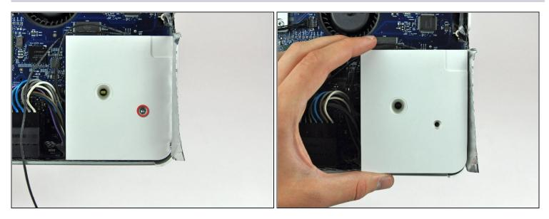
• Remove the single T10 Torx screw securing the right speaker to the rear case.
