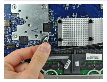
• De-route the IR cable from under the aluminum heat sink and tuck it behind the optical drive to keep it out of the way.
