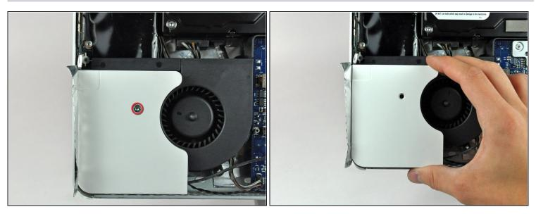
• Remove the single T10 Torx screw securing the left speaker to the rear case.
