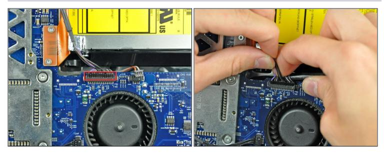
• Disconnect the IR/camera cable from the logic board.
