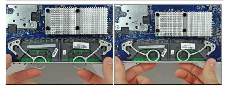
• Tuck the RAM arms into the iMac so they rest on the perforated metal grille along its lower edge.
