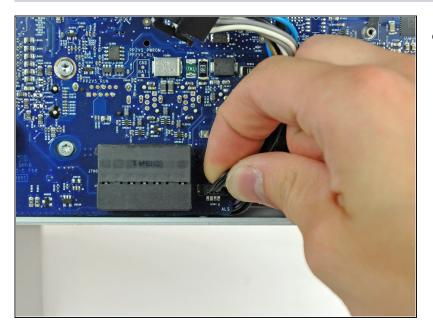
• Disconnect the ambient light sensor by pulling its connector away from the face of the logic board.
