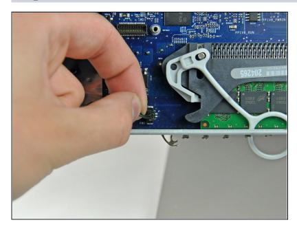
• Disconnect the power button cable by pulling its connector away from the face of the logic board.
