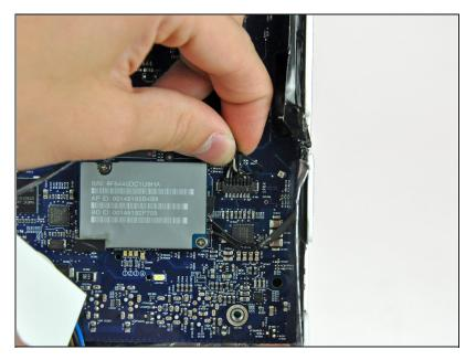
• Disconnect the speakers from the logic board by pulling their connector toward the top edge of the iMac.
