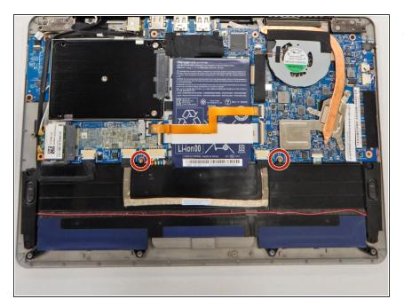
With the Phillips #0 screwdriver, remove the two 5 mm screws that are located above the long black piece of the battery.
