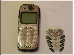
Lightly peel the keypad off of the phone.
