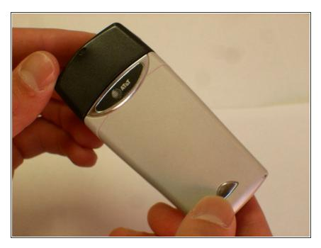
Locate the button on the bottom of the back cover.
