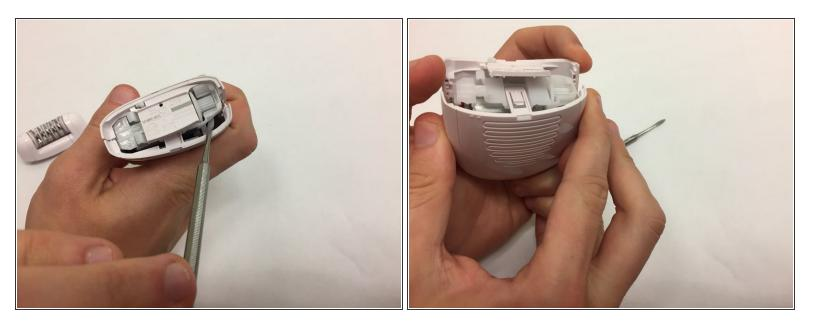
• Use a metal spudger to pry open the casing.
