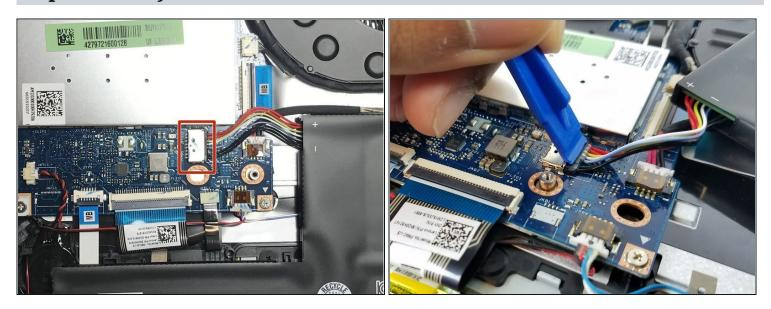
• Disconnect the battery by using a plastic opening tool or your fingers to push the connector towards the battery.
