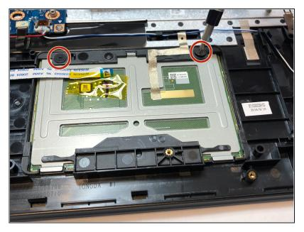
• Locate the touch pad and remove the two 3 mm screws using a T5 Torx Screwdriver.
