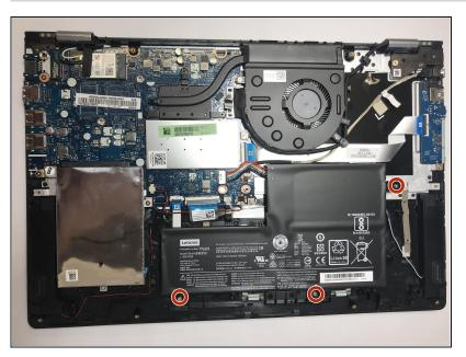
• Remove the three 4 mm screws using a T5 Torx Screwdriver.
