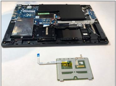
• Open the laptop and, with the assistance of the iFixit blue plastic tool, guide the touch pad through, it should come out on its own.
