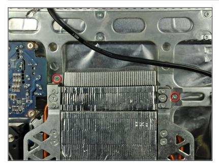
Remove the two T6 Torx screws near the top of the heat sinks.
