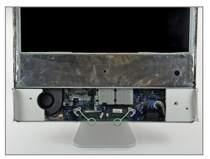
Tape the lower EMI shield up against the face of the display to keep it out of the way while you work.
