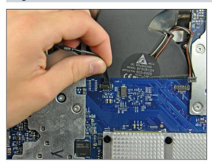
Disconnect the hard drive thermal sensor from the logic board by pulling its connector toward the top edge of the iMac.
