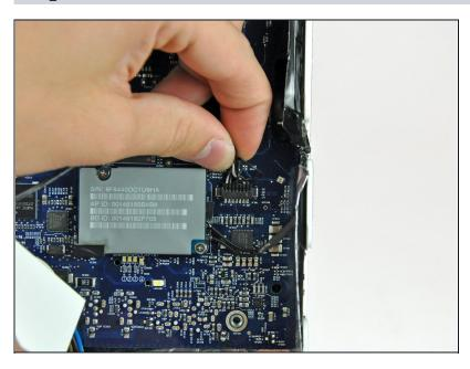
Disconnect the speakers from the logic board by pulling their connector toward the top edge of the iMac.
