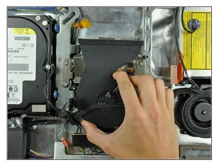
Lift the CPU fan off the plastic posts protruding from the rear case.
