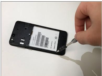
Remove the sixteen 3mm screws using the Phillips #000 screwdriver.
