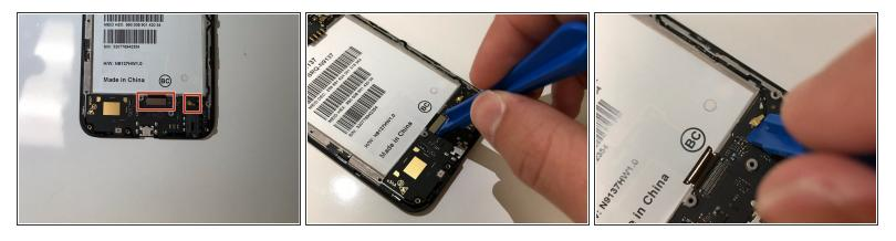
• Using a spudger, unclip the board from the phone at the places highlighted.
