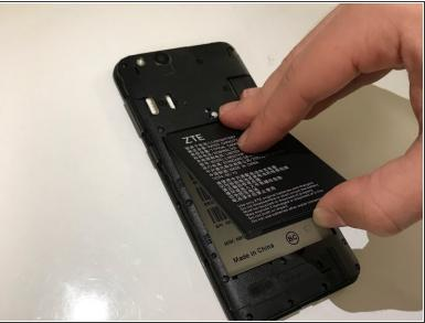
• Find the divot near the bottom of the battery and remove the battery from the device.
