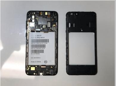
Take off the second back cover, lifting from the bottom of the device to the top.
