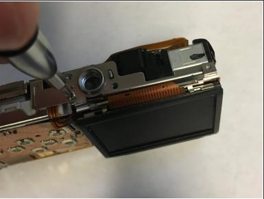
Remove screws both at the top and the base of the screen to free the screen.
