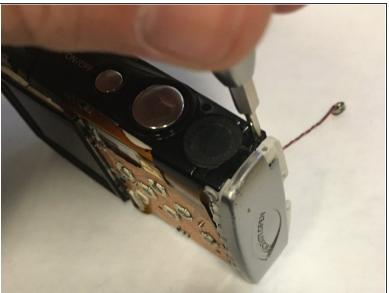
Remove top button panel by removing the screw located at the top right of the panel.
