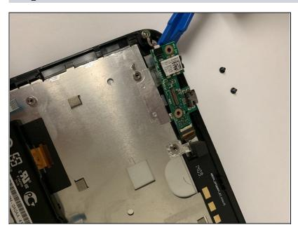
Pull the board up using the opening tool.
