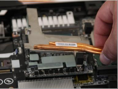
Unscrew the CPU cooling plate using the Phillips #0 screwdriver. Lift the cooling pipes away from the unit. Screws are 0.15625 inches long.
