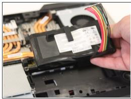
Unplug the battery plug from the unit. Lift the battery out of the housing by prying it from the adhesive using the black nylon spudger.
