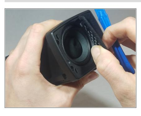
Using your fingers, lift up on the end cap cover until it separates completely from the main body of the device.
