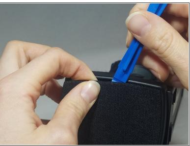
Using the blue plastic opening tool, pry up on the cloth covered end panel. The edge of end cap cover should separate from main body of device.
