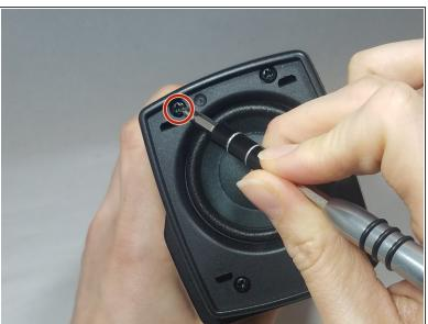
Remove the 4, PH1, 15mm screws on the side speaker cover frame.
