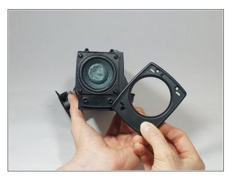
Remove speaker cover frame from main body of device.
