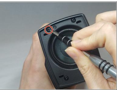
• Remove the 4, PH1, 15mm screws on the side speaker cover frame.
