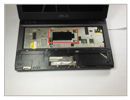
if you want to add additional RAM, more ports can be found underneath the black plastic flap on the top side of the laptop, just under the keyboard. These ports behave the same way as the ones on the backside of the computer.
