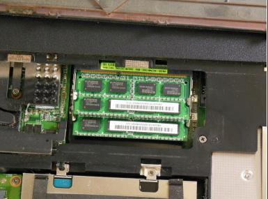
With the underside plate removed, you can easily access a few RAM chip slots. These are the ones most likely filled with RAM chips from the factory when purchased at retail.
