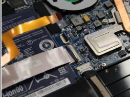
Remove the motherboard connector cables by gently lifting the black latch that clamps them in place with a spudger or simply pull the connector from the port.
