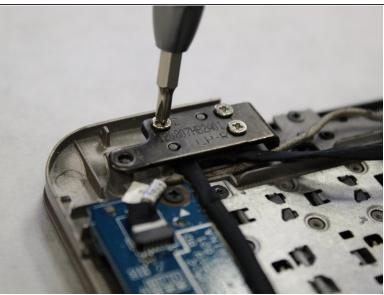
Unscrew the 10 5mm PH00 screws from the hinges attaching the display assembly to the base.
