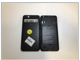
Pry open back cover of the device from the crease at the bottom left corner with an opening tool or fingernail.
