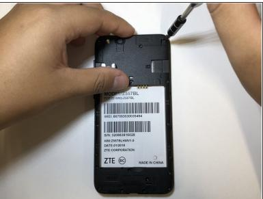
Remove all 16 screws with a J000 screwdriver.
