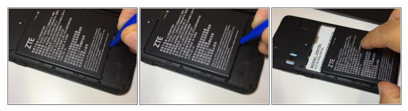
Remove the battery with an opening tool or fingernail.
