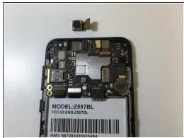
Using the blunt-nose tweezers, tug at the camera gently, switching sides to remove adhesive little by little, pull camera out gently.
