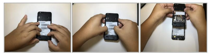
Gently pry open the device body by tugging from the inside out, be sure to pull up and away from device.
