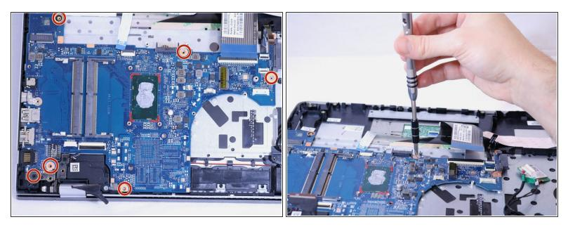
Use a PH1 screwdriver to unscrew six 3 mm Phillips head screws on the motherboard.
