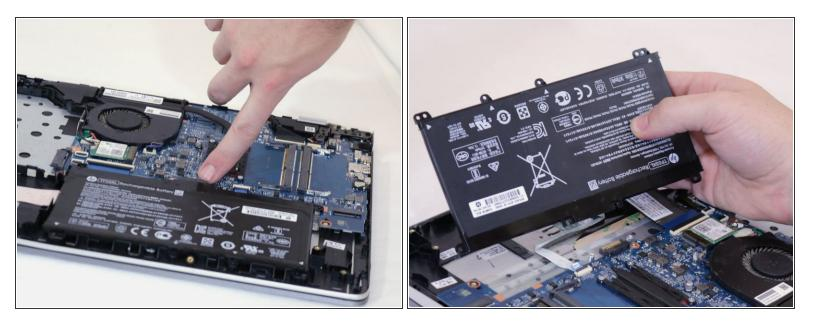
Disconnect the port connecting the battery and the motherboard and then remove.
