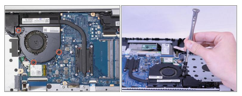
• Use a PH0 screwdriver to unscrew the three 3 mm Phillips head screws located on the fan.
