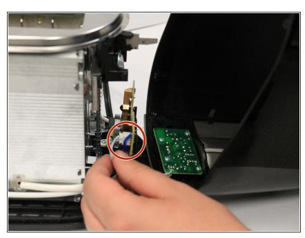
To detach the bundled cable connector, carefully pull it away from the circuit board.
