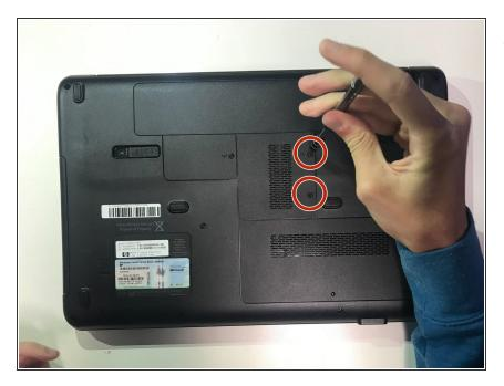
Using a standard #2 Phillips-head screwdriver, remove the back compartment of the CQ60 to access the motherboard.
