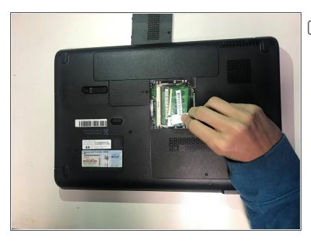
Carefully insert the new RAM, and ensure that it is placed in the correct slots.
