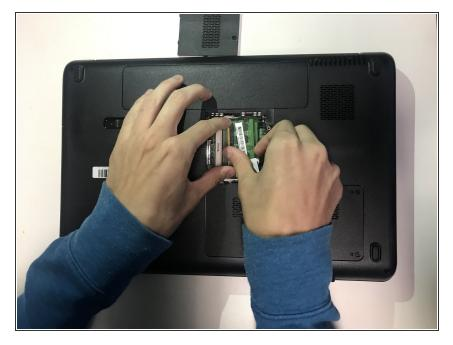
Use your fingers to push the retention clips away from the RAM sticks, and carefully pull out the old RAM.
