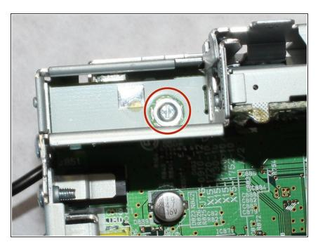
Remove the 5mm screw with a Phillips #1 screwdriver.
