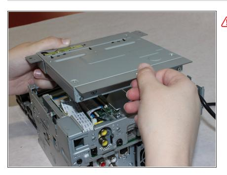
⚠ Lift the CD drive carefully to expose the attached cable underneath.
