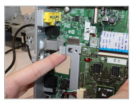
To remove and reinsert the connector, on the top side of the board, use your finger to gently lift the metal plate to get enough clearance.
