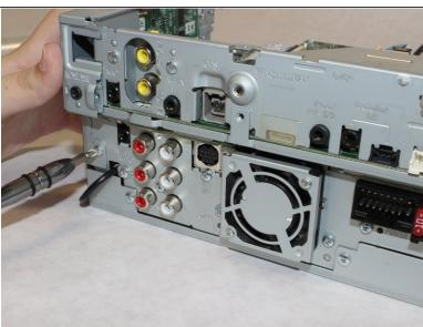
Unscrew the three 5.5mm long screws with a Phillips #1 screwdriver.
