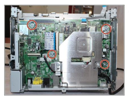
Remove the four 5mm screws with a Phillips #1 screwdriver.
