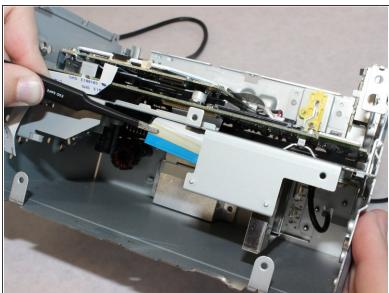
Using a spudger, undo the clasp to disconnect the large white ribbon cable.
