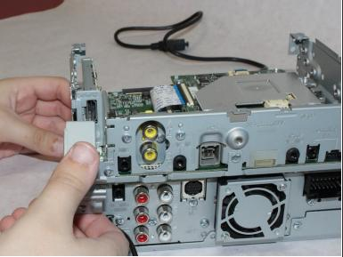
• Remove the 5.5mm screw from the HDMI cable cover using a Phillips #2 screwdriver.
