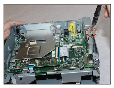
Remove the 5mm screw with teeth from the casing with a Phillips #1 screwdriver.
